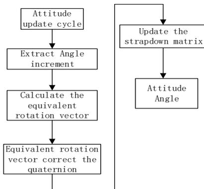
Figure.2 Calculation procedure of equivalent rotation vector method
