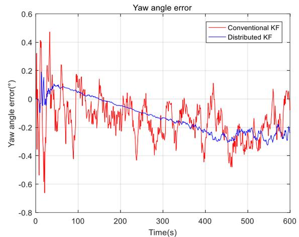
Figure.7 Yaw angle error comparison diagram
