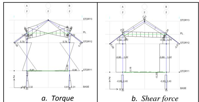
Figure 3. Internal force in beams, column with wall construction in horizontal direction of the house
