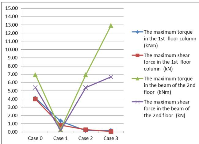
Figure 6. Comparison of shear and torque forces in columns, beams on the 1st and 2nd floor in the cases
