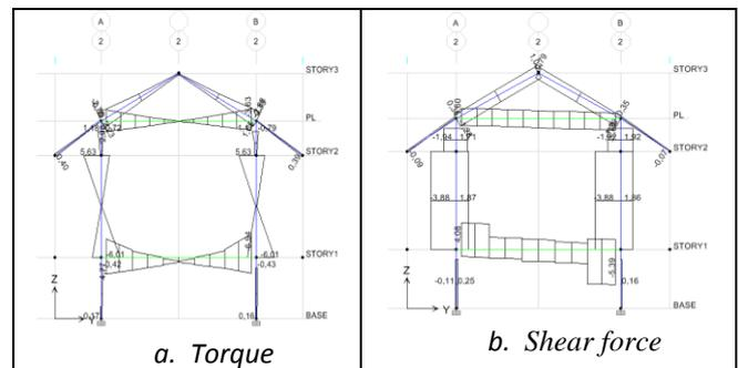
Figure 4. Internal force in beams, columns with forced anti-oblique addition along the house
