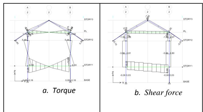
Figure 5. Internal force in beams, columns with reinforced walls on both sides of columns
