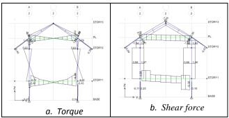
Figure 4. Internal force in beams, columns with forced anti-oblique addition along the house
