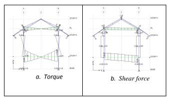
Figure 5. Internal force in beams, columns with reinforced walls on both sides of columns
