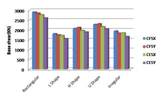
Figure 8. Base shear of buildings in X direction, Y direction with CFS and CES columns.
