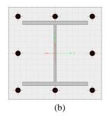
Figure 6. Filled concrete a) Concrete filled steel b) Concrete encased steel I section
