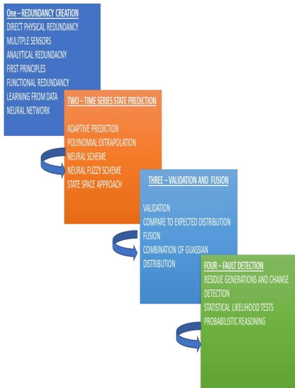
**Figure 5: Flow chart representation of the four steps of the methodology along with tools**
