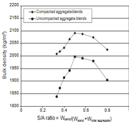
Fig. 2. Bulk density of different aggregate blends
