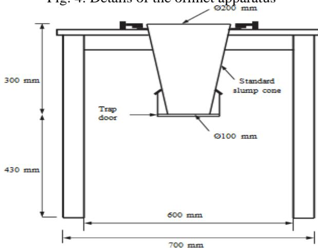
Fig. 5. Details of the inverted slump cone apparatus
