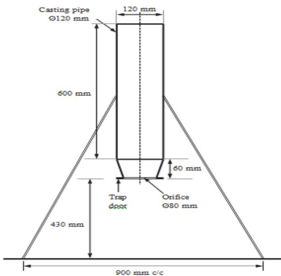
Fig. 4. Details of the orimet apparatus
