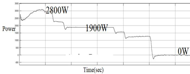
Figure 12: Active power injected to the grid by string PV inverter system
