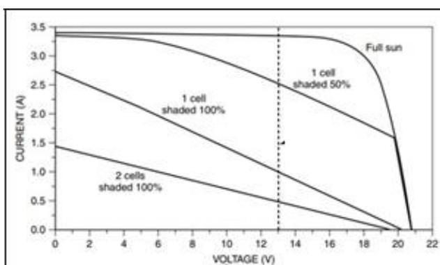
Figure 1: Shading effect on Solar cell
