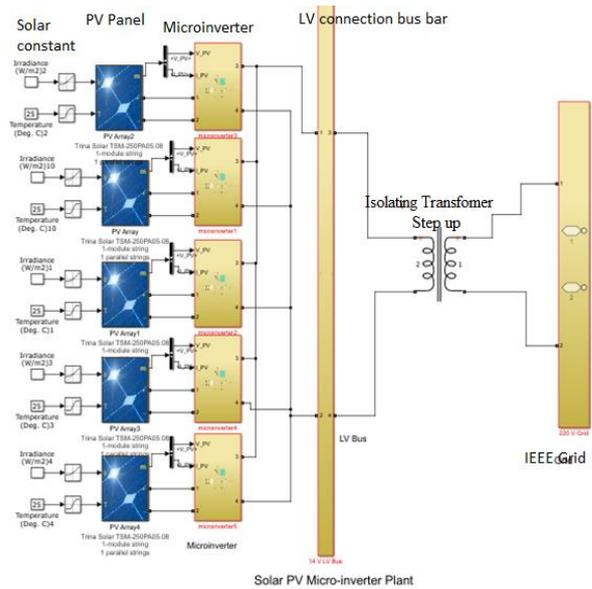
Figure 10: Parallel Microinverter system with line transformer
