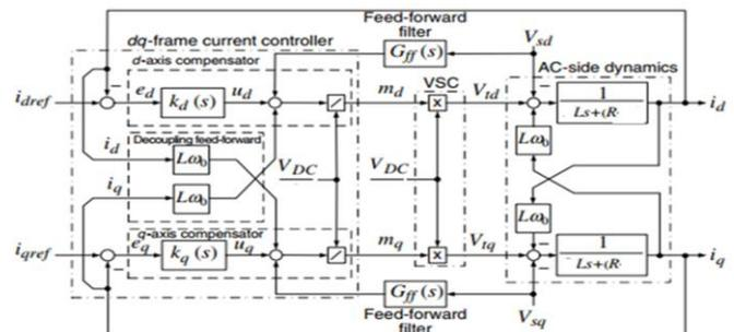
Figure 4: Current control algorithm for grid connected system
