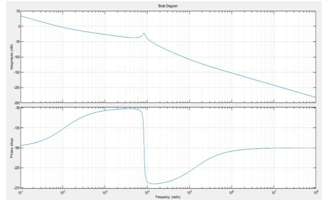
Figure 6: Bode plot of LCL parameter after K and Ki tuning
