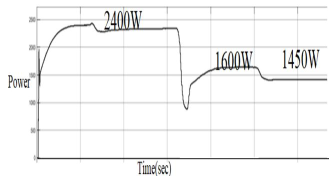
Figure 11: Active power injected to the grid by microinverter system
