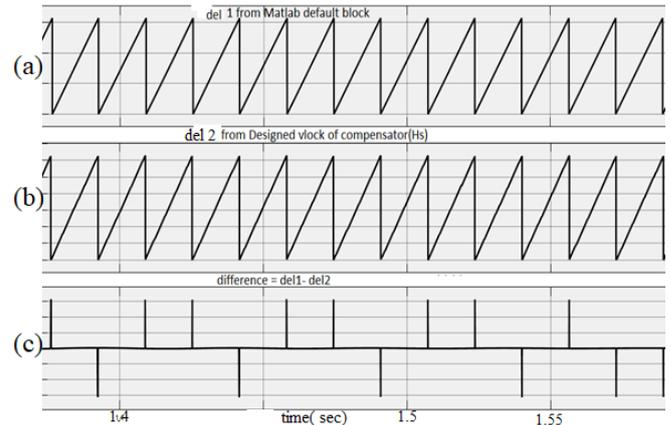
Figure 2: (a) MATLAB default PLL, (b) designed PLL and (c) its error
