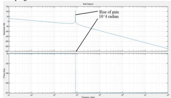
Figure 7: Bode plot when damping resistance, Rd = 0
