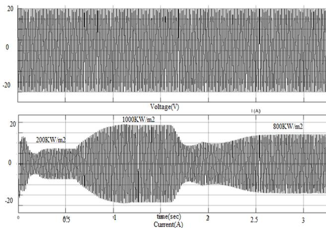
Figure 9: Voltage and current of inverter in grid connected mode with changing irradiance
