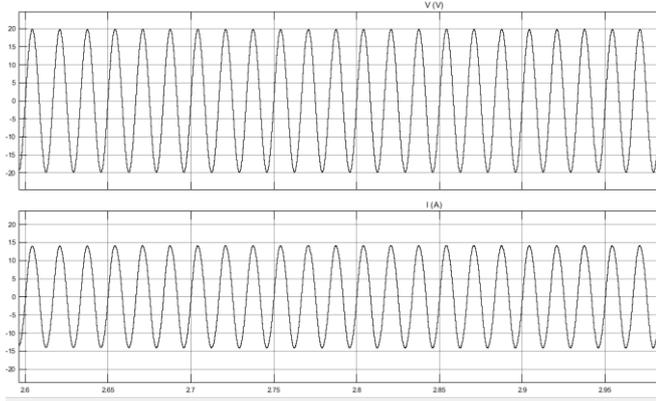
Figure 8: Sinusoidal voltage and current profile from 2.6 sec to 3 sec at  $800\text{W/m}^2$
