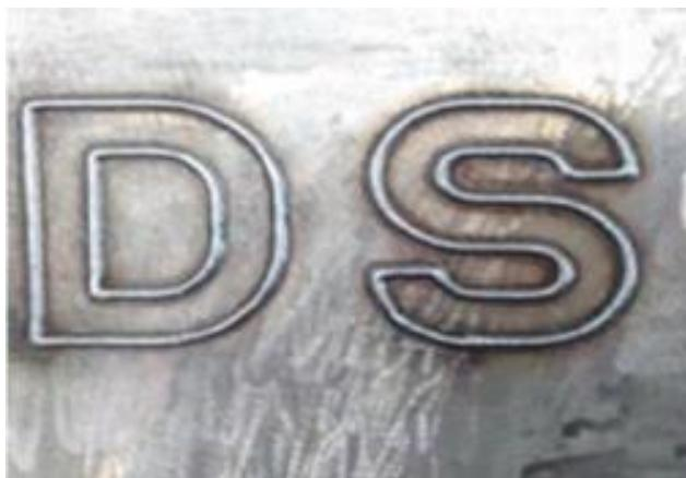
Figure 9 hull marker word "D, S" welding
