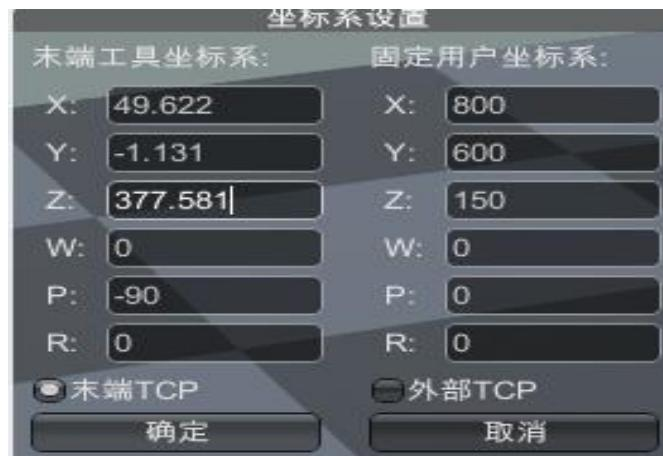
Figure 6 Tool and workpiece coordinate system parameter settings
