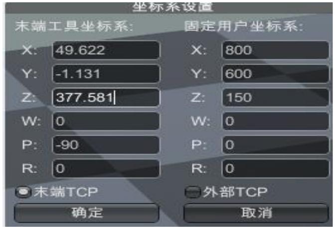
Figure 6 Tool and workpiece coordinate system parameter settings
