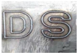
Figure 9 hull marker word "D, S" welding
