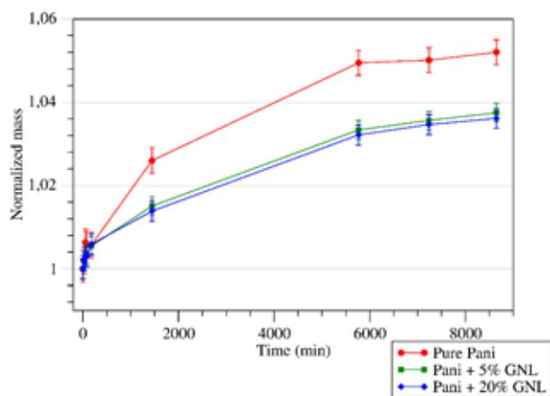
Fig. 6 – Time evolution of the mass of polyaniline samples containing different amounts of GNL and exposed to air. The lines are only to guide the eyes.
