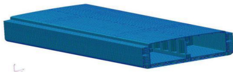
Fig 1 Temperature field calculation finite element model.
