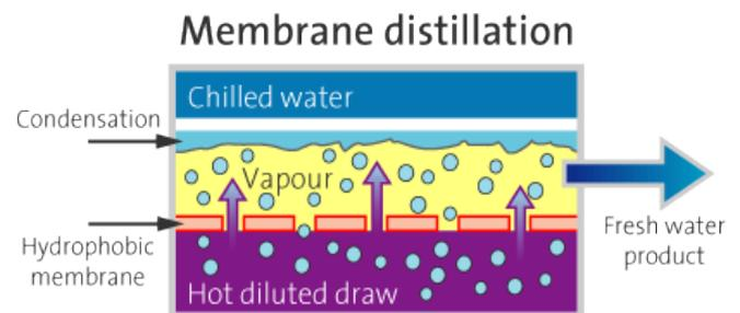
Fig. 3. Principle of MD separation process [15].
