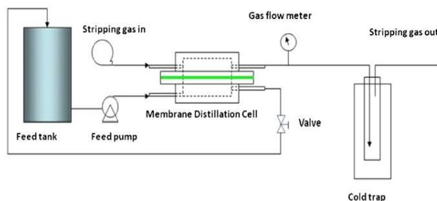
Fig. 8. Gas stripping electro-spun nanofiber MD system [22].
