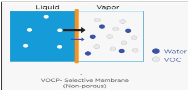
Fig. 1. Pervaporation mechanism in the treatment of VOCs from water [12].
