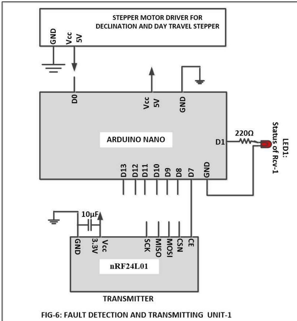
FIG-6: FAULT DETECTION AND TRANSMITTING UNIT-1
