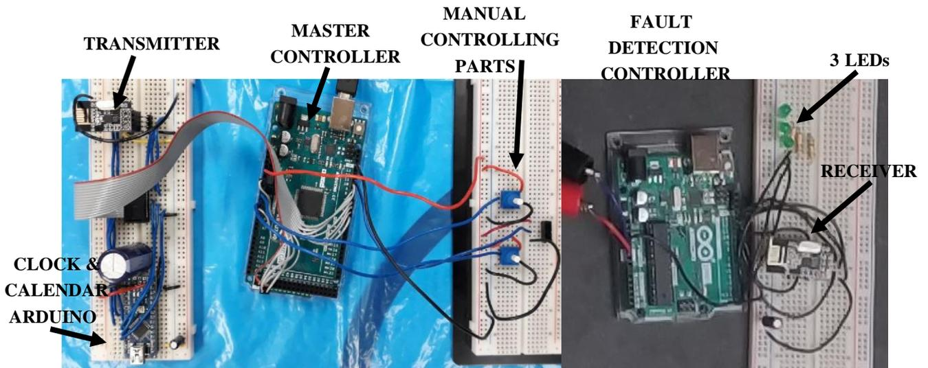
FIG. 9 - A PHOTOGRAPH OF THE EXPERIMENTAL SETUP – MAIN CONTROL ROOM
