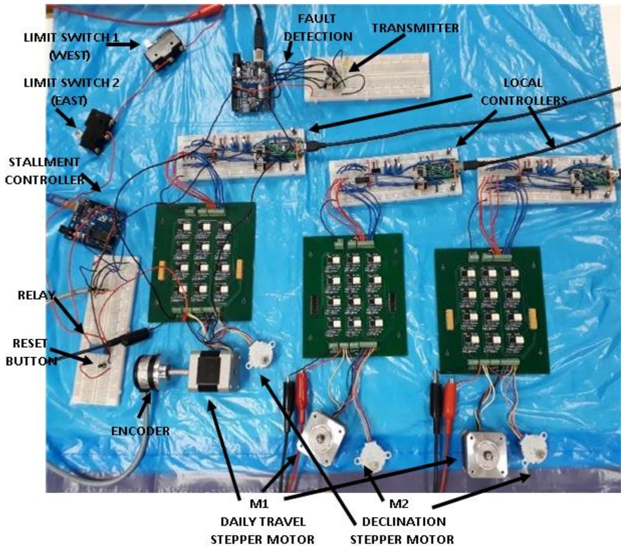
FIG.10 A PHOTOGRAPH OF THE EXPERIMENTAL SETUP WITH INDIVIDUAL MACHINES
