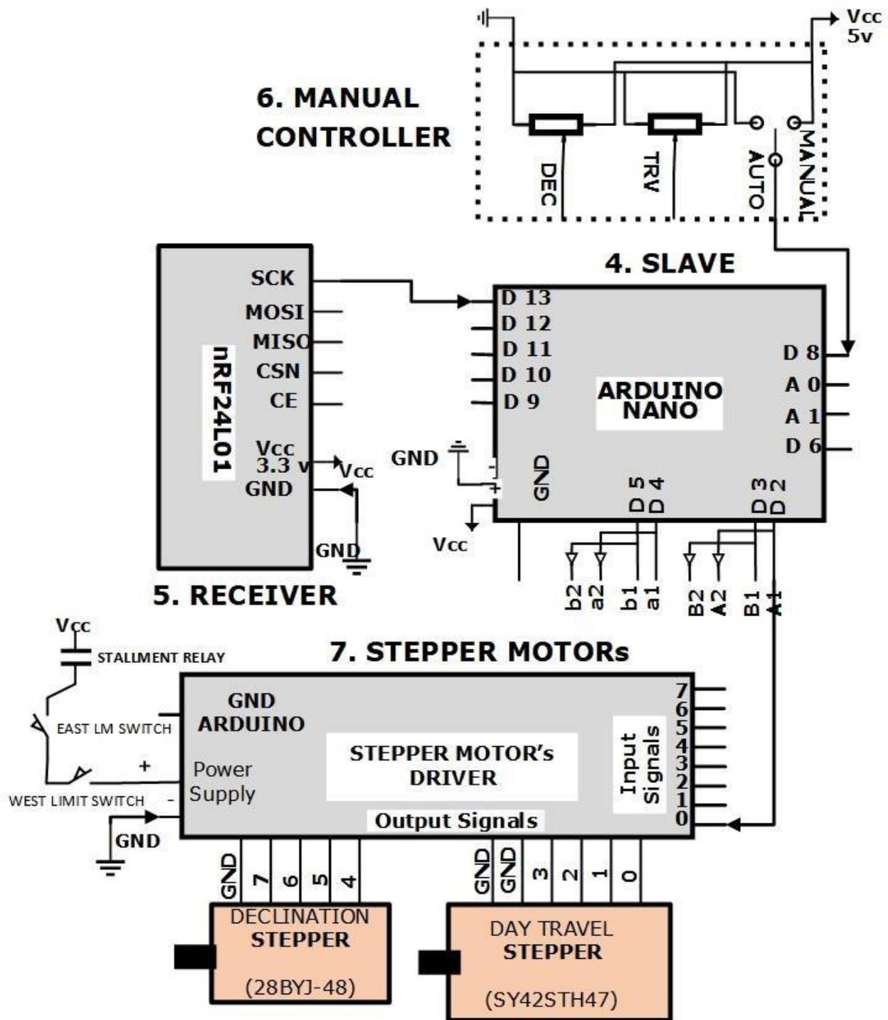
FIG. 5 – CIRCUITRY AT THE MACHINE LEVEL
