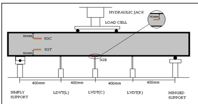
Fig. 1 Experimental Setup of RC beam for testing
