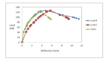
Fig.5(c) Load Vs Deflection of FSW-F specimen
