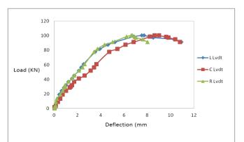
Fig.5(a) Load Vs Deflection of FCB specimen
