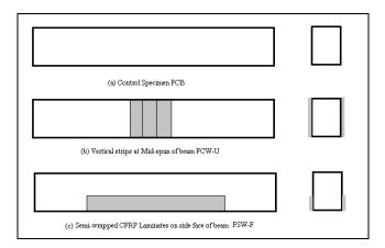
Fig.3 Wrapping of CFRP laminates
