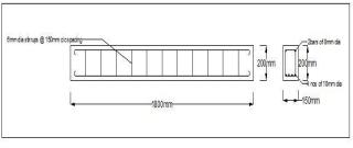
Fig. 2 Reinforcement details of beam
