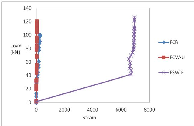
Fig.8 Load Vs Bottom Strain for all specimen
