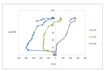
Fig.7(a) Load Vs Strain for FCB specimen
