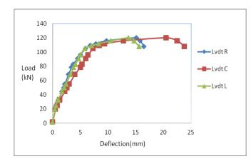
Fig.5(b) Load Vs Deflection of FCW-U specimen
