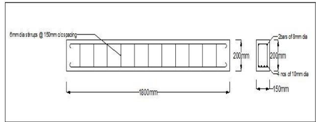
Fig. 2 Reinforcement details of beam
