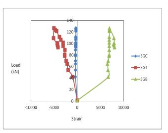
Fig.7(c) Load Vs Strain for FSW-F specimen
