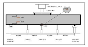
Fig. 1 Experimental Setup of RC beam for testing
