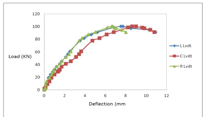
Fig.5(a) Load Vs Deflection of FCB specimen
