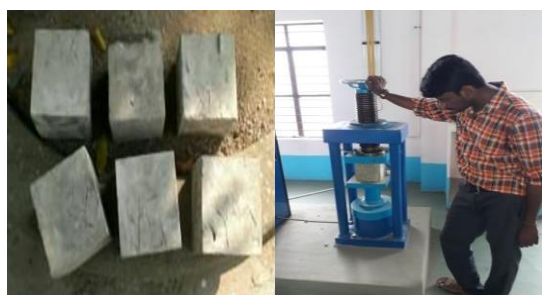
Compressive Strength Results for M30grade Concrete With Various % Of Partial Replacement of GGBS &10% PLASTIC for 7,14,28,56 days
