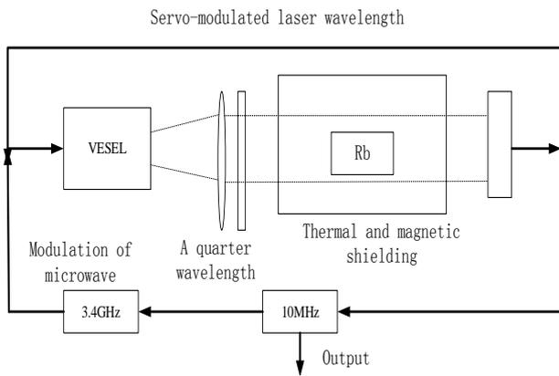
Figure 1 CPT atomic clock working principle diagram
