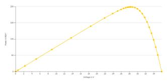
Fig 3. P-V curve of PEPV\_48 200W at standard condition (1000W/m², 25  $^{\circ}\mathrm{C})$
