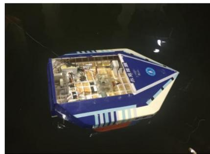
Fig 1.4 Rolling Attenuation Test of Small Waterplane Area Quad-Hull-USV in Still Water
