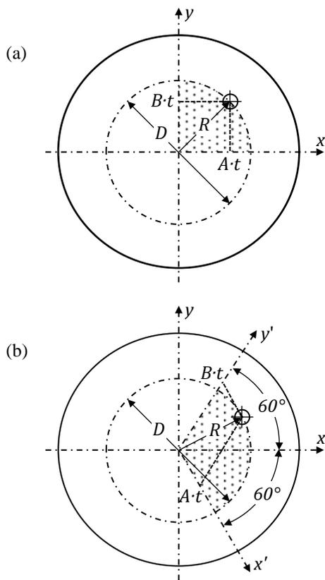
Fig. 3: Axes and coordinates, (a) for square pattern SQ-1, (b) for triangular pattern TR-1
