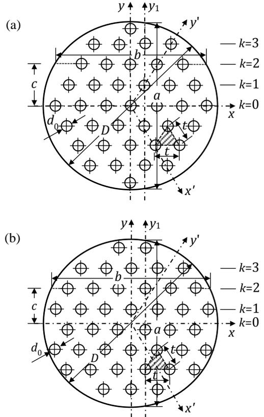
Fig. 2: Triangular pattern, (a) with a hole at the center (TR-1), (b) without a hole at the center (TR-2)
