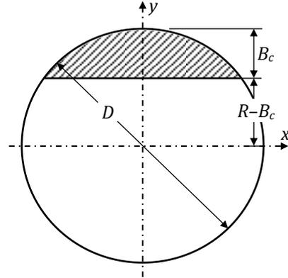
Fig. 5: Segmental baffle geometry
