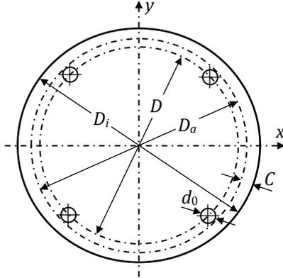
Fig. 4: Geometry of a tube-sheet
