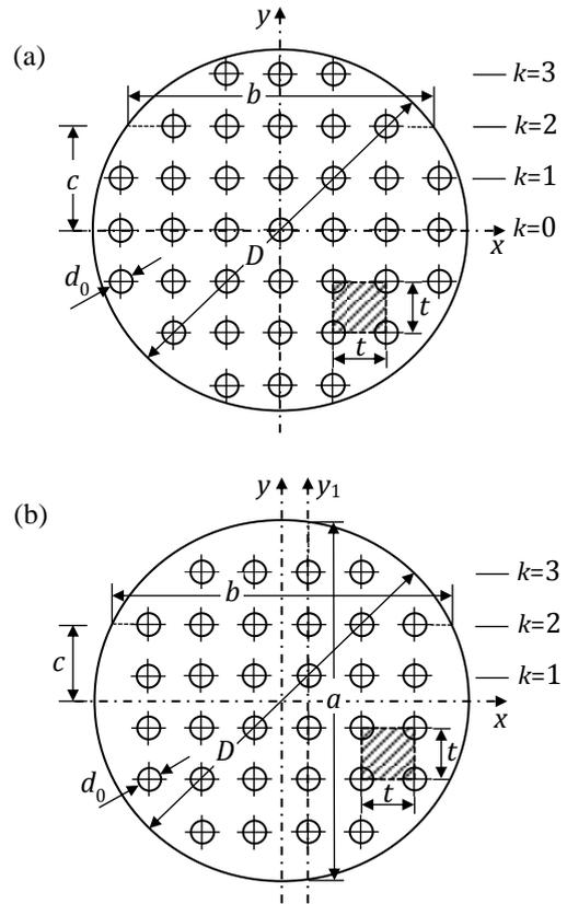
Fig. 1: Square pattern, (a) with a hole at the center (SQ-1), (b) without a hole at the center (SQ-2)
