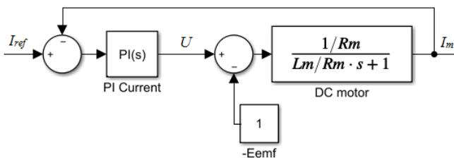
Fig. 3: Closed-Loop DC motor current Control System
