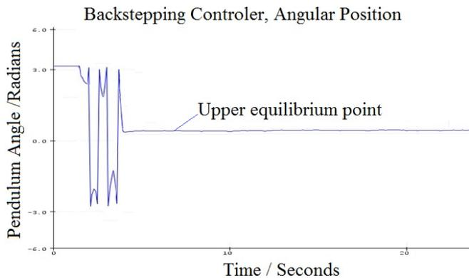
Fig. 12: Experimental Swing-Up & Stabilization using Backstepping control
