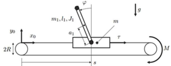
Fig. 2: Reference frames and parameters of pendulum
