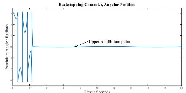
Fig. 9: Simulation of Swing-Up & Stabilization using Backstepping control
