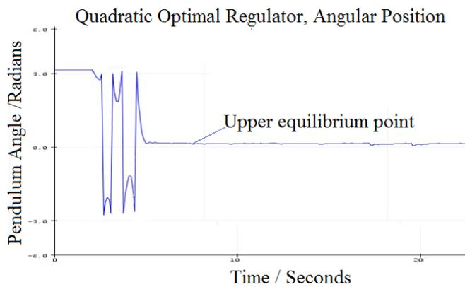
Fig. 11: Experimental Swing-Up & Stabilization using Quadratic Optimal Regulator
