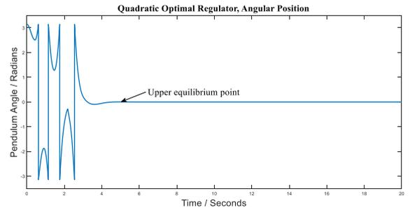
Fig. 7: Simulation of Swing-Up & Stabilization using Quadratic Optimal Regulator
