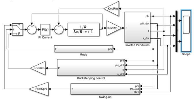
Fig. 8: Block diagram of controller using backstepping control
