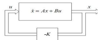
Fig. 5: Block diagram of the optimal regulator system
