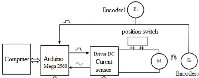
Fig. 10: Block diagram of experimental setup
