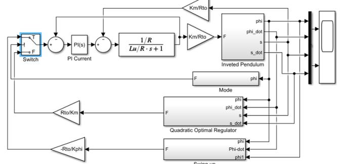
Fig. 6: Block diagram of controllers using Quadratic Optimal Regulator (MATLAB Simulink).
