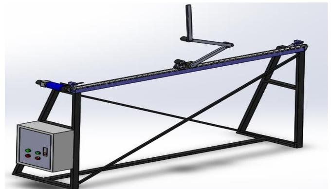
Fig. 13: 3D Solidworks Triple inverted pendulum system
