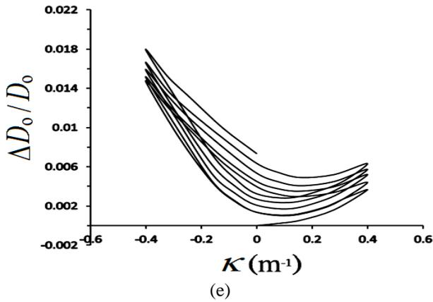
Fig. 6 Experimental ovalization ( $\Delta D_0/D_0$ ) - curvature ( $\kappa$ ) curves for local sharp-dented 6061-T6 aluminum alloy tubes with  $a =$  (a) 0.0, (b) 0.3, (c) 0.6, (d) 0.9 and (e) 1.2 mm under cyclic bending
