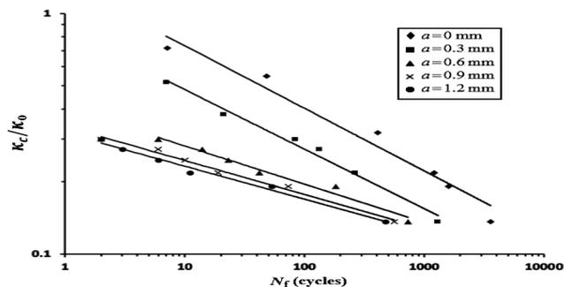
Fig. 8 Experimental cyclic curvature ( $\kappa_c/\kappa_0$ ) versus the number of bending cycles required to ignite failure ( $N_f$ ) for local sharp-dented 6061-T6 aluminum alloy tubes with different  $a$ s on double logarithmic coordinates
