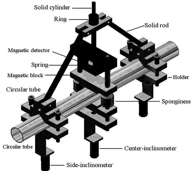
Fig. 3 A schematic drawing of the curvature-ovalization measurement apparatus
