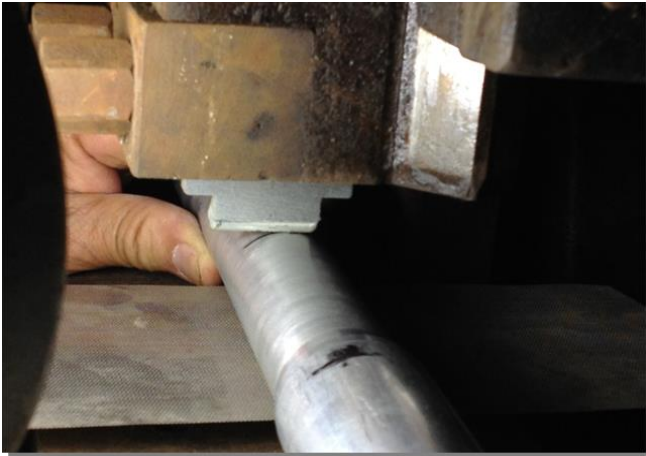
Fig. 3 A picture of processing a sharp dent on the 6061-T6 aluminum alloy tube
