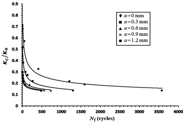
Fig. 7 Experimental cyclic curvature ( $\kappa_c/\kappa_0$ ) versus the number of bending cycles required to ignite failure ( $N_f$ ) for local sharp-dented 6061-T6 aluminum alloy tubes with different  $a$ s on decimal coordinates
