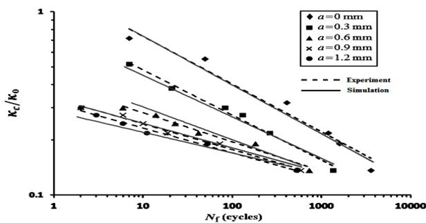
Fig. 11 Experimental and simulated cyclic curvature ( $\kappa_c/\kappa_0$ ) versus the number of bending cycles required to ignite failure ( $N_f$ ) for local sharp-dented 6061-T6 aluminum alloy tubes with different  $a$ s on double logarithmic coordinates
