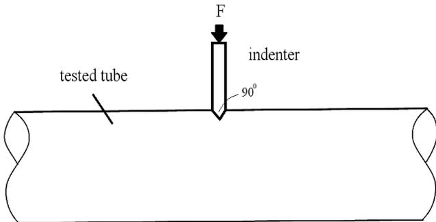
Fig. 4 A schematic drawing of processing a sharp dent on the 6061-T6 aluminum alloy tube
