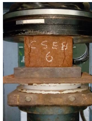
Fig 1. CSEB saturated blocks tested in CTM
