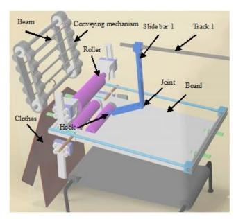
Figure 2. New type of folding machine
