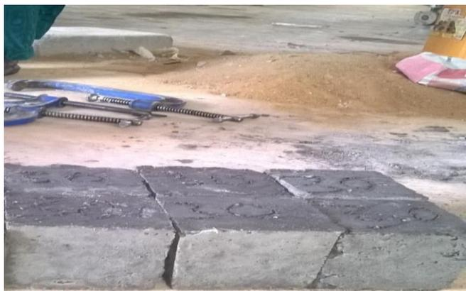
Plate IX: CONCRETE CUBES FROM LBWA CONTAINING 30% CEMENT REPLACEMENT
