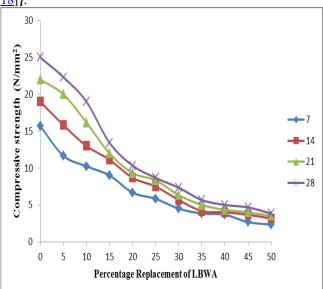
Fig. 5: Variation of concrete compressive strength with LBWA replacement of cement at different curing age
