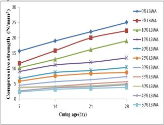
Fig. 4: Variation of concrete compressive strength with age at different percentages of cement replacement with LBWA
