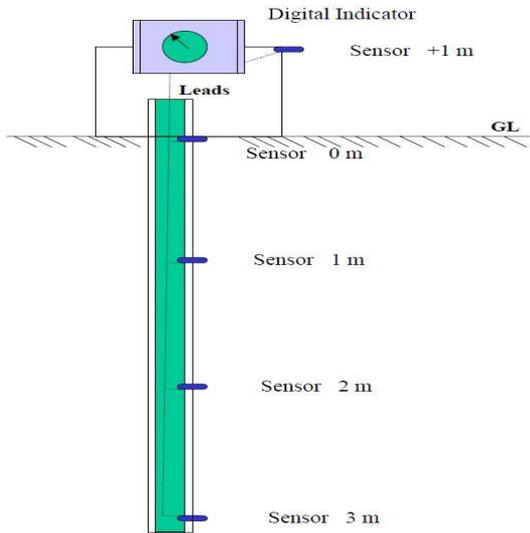
Figure 1: Thermocouple placement into the tube at different ground level
