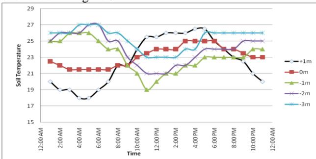
Figure 3: Soil temperature at various depths and ambient Temperature at KUET campus, Khulna at 23rd December 2008
