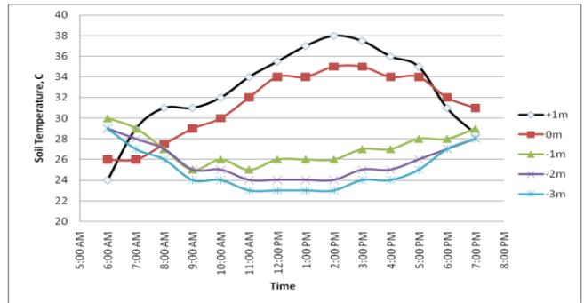
Figure 4: Ground temperature at various depths and ambient temperature at KUET campus, Khulna at 19th April 2008
