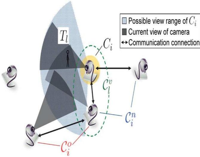
Fig. 1. Conceptual illustration of camera network topologies.  $\mathcal{C}_i$  is the subset of all cameras viewing target  $l$  and the rest of the cameras are  $\mathcal{C}_{-i}$ .  $\mathcal{C}_i^n$  is the set of neighboring cameras of  $i$  and defined as all the cameras with which  $i$  is able to communicate.  $\mathcal{C}_i^o$  is the set of overlapping cameras of  $i$ , and is defined as all the cameras with which  $i$  can potentially have an overlapping field of view.
