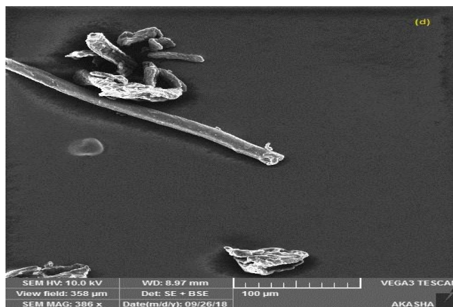
Figures13d. SEM image of synthesized CMC by 35 g/dL NaOH.
