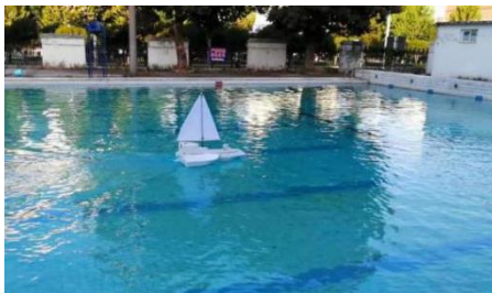
Figure 2 Three-body rescue unmanned craft surface navigation test
