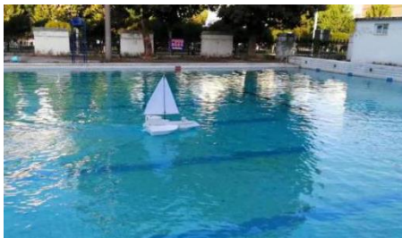
Figure 2 Three-body rescue unmanned craft surface navigation test
