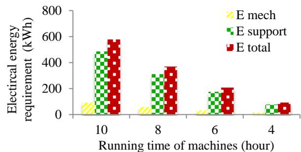
Fig.7 Electrical energy consumption with drying time
