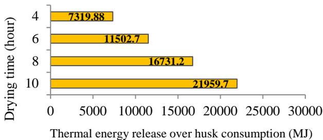
Fig. 9 Thermal energy from rice husk with respect to drying time
