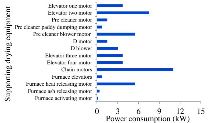
Fig.6 Power consumption of supporting equipments
