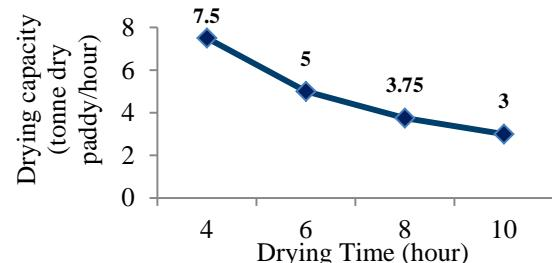
Fig.11 Drying capacity with drying time
