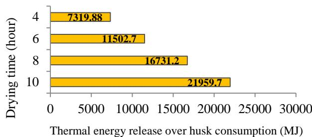
Fig. 9 Thermal energy from rice husk with respect to drying time
