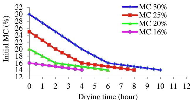
Fig.10 Moisture losses of paddy with drying time
