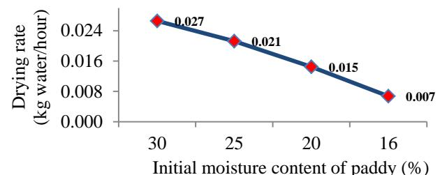
Fig.12 Drying rate with initial MC of paddy
