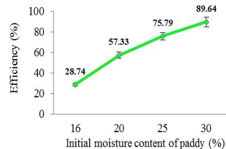
Fig. 13 Drying efficiency with Initial MC of Paddy
