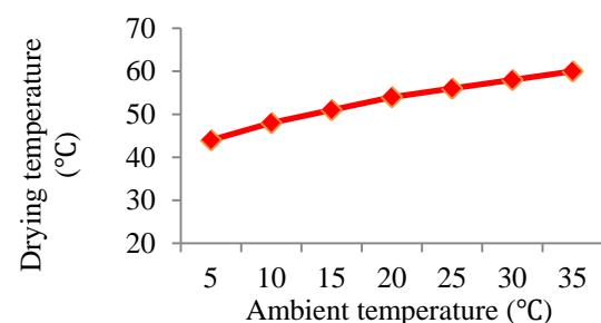
Fig.4 Relationship of drying temperature and ambient temperature
