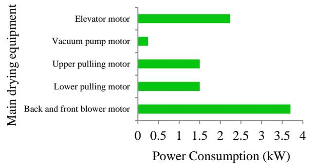
Fig.5 Power consumption of main drying equipments
