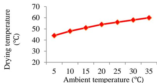
Fig.4 Relationship of drying temperature and ambient temperature
