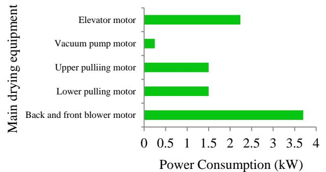
Fig.5 Power consumption of main drying equipments
