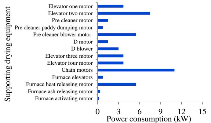
Fig.6 Power consumption of supporting equipments
