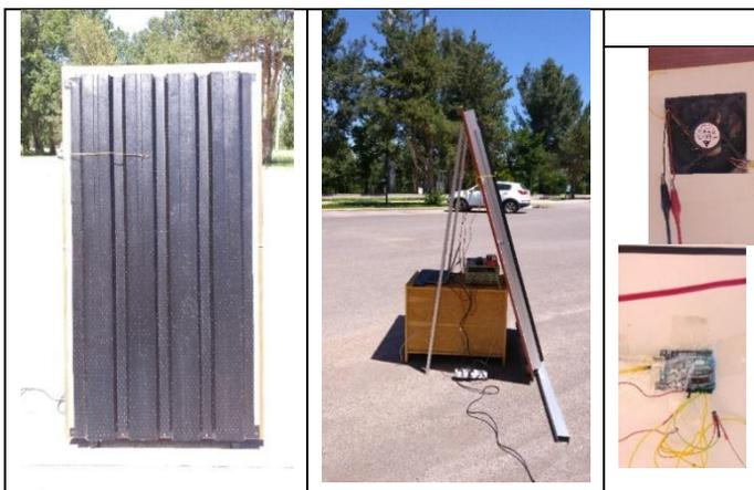
Figure 2. Experimental setup of the UTC air heating system.
