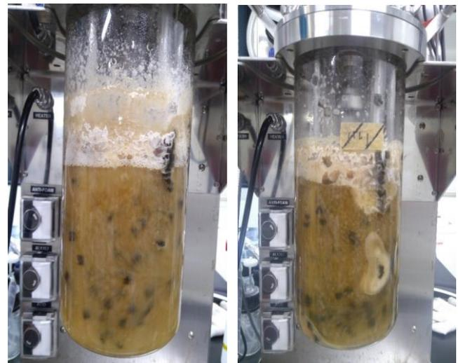
Fig. 4. (a) Uniform distribution of 500 large -BSPs at  $t = 48h$ ; (b) Preparation of a dead-mixing zone in the tank wall caused by increase in the number of BSPs, (1,000 -large BSPs) at  $t = 48 h$ .
