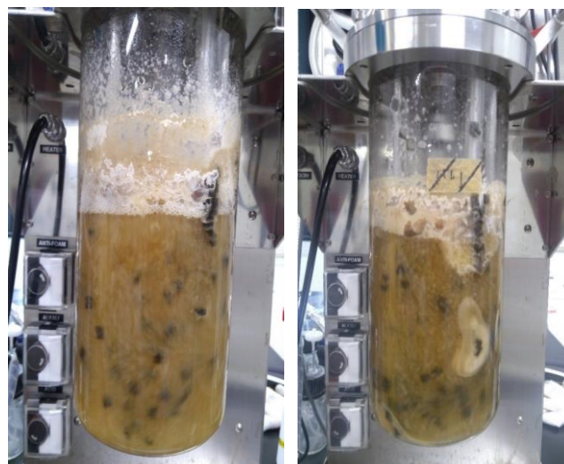
Fig. 4. (a) Uniform distribution of 500 large -BSPs at t = 48h ; (b) Preparation of a dead-mixing zone in the tank wall caused by increase in the number of BSPs, (1,000 -large BSPs) at t = 48 h .
