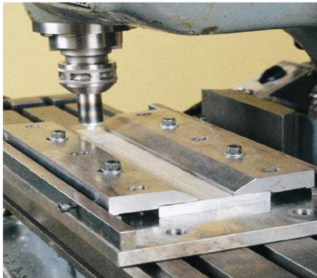
Fig.1. Friction stir Welding process
