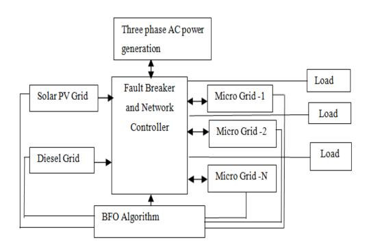
Figure.1.Functional Block Diagram of the System
