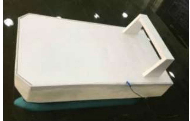
Figure 2 Hydro static pitching attenuation test of SWATH
