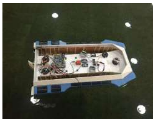
Figure 3 Two-body unmanned boat static water pitch attenuation test
