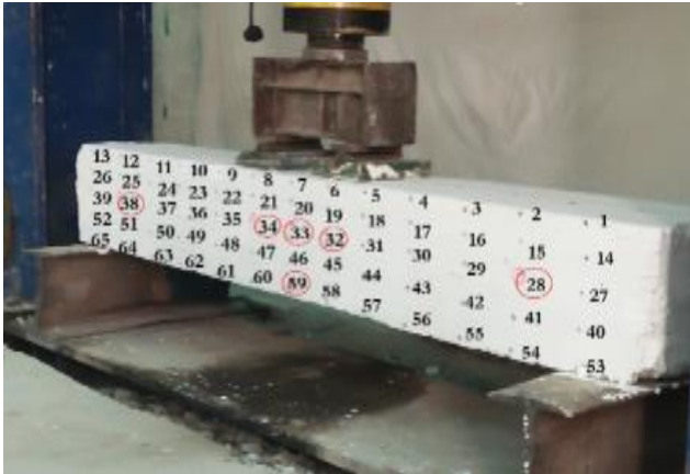
Fig (4) monitoring point on the beam
