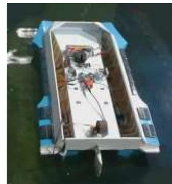
Fig.2.2 Hydrostatic roll attenuation test for catamaran unmanned craft in still area
