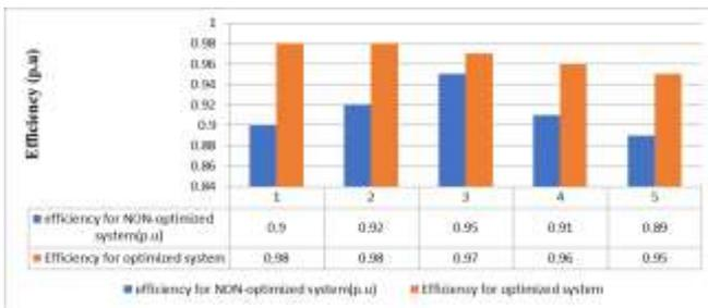
Fig 12.0: Comparison of efficiency for both drive systems
