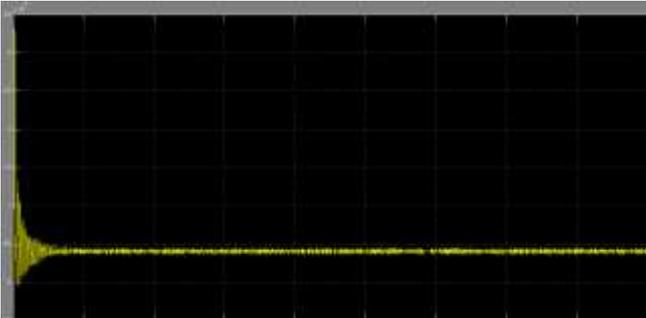
Fig 11.0: Input power of a drive system without controller
