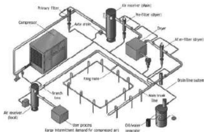
**Fig 2.0:** Typical compressed air system (source: Carbon Trust 2005)
