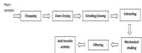
Fig. 2 A diagram showing the overall process steps of hydro-alcoholic extraction from wild giant taro
