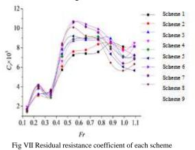
We can see from Figure VII, the residual resistance coefficient increase with increase of Froude number, showed the trend of increasing firstly and then decreasing, and the scheme 6 and 9 in the Froude number of 0.82, show better performance of resistance.
