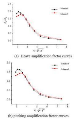
Fig. VIII curve of seakeeping performance
