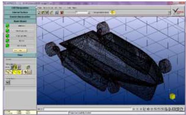
Fig VI Mesh model of amphibious ship
