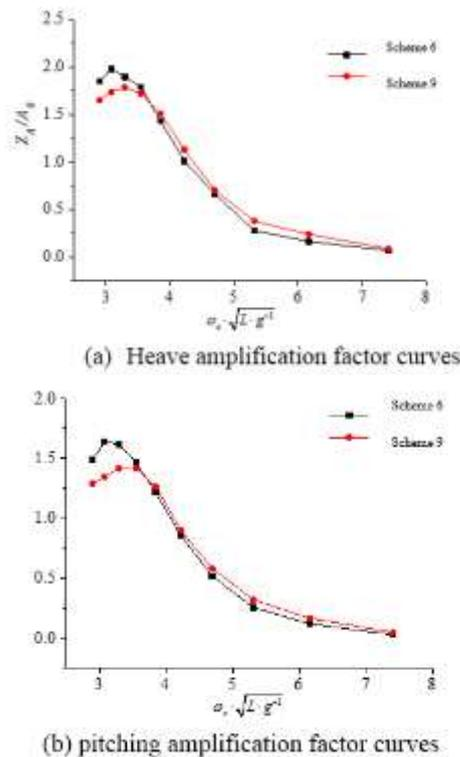
Fig. VIII curve of seakeeping performance
