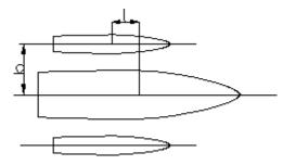
Fig. V Sketch map of relative positional parameters of trimaran's main and side body
