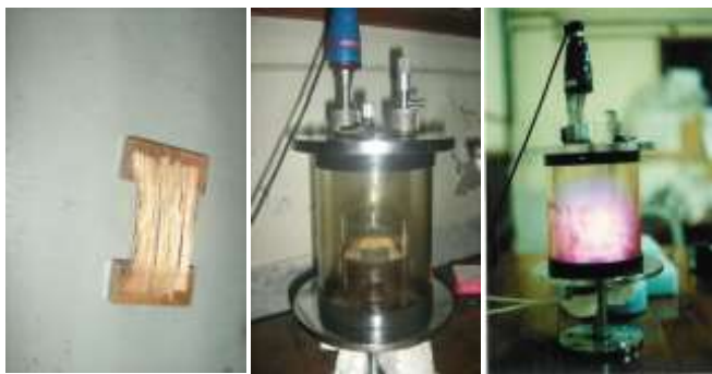
Fig. 1 Schematic diagram of jute fibre and position of it in the glow discharge reactor
