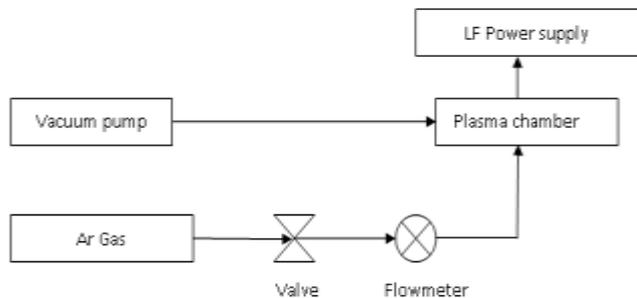
Fig. 2 Flow chart of the plasma treatment set-up
