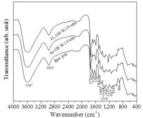
Fig. 8 FTIR spectra of raw, Ar and O<sub>2</sub> LTP treated jute at 100 W, 15 min.
