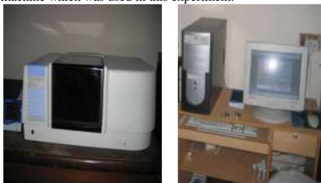
Fig. 3 A photograph of a FTIR spectrometer
