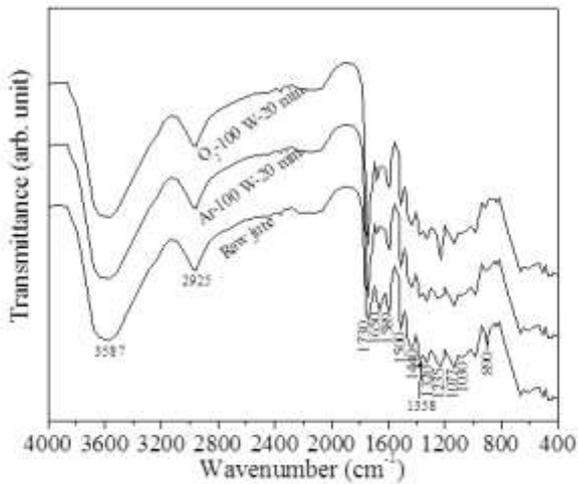
Fig. 6 FTIR spectra of raw, Ar and O<sub>2</sub> LTP treated jute at 100 W, 20 min.
