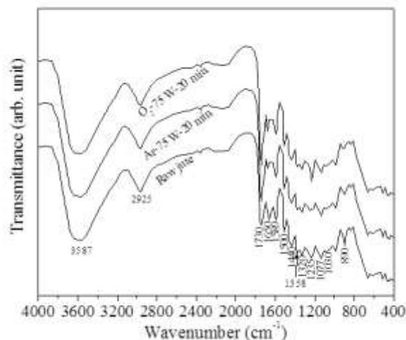
Fig. 5 FTIR spectra of raw, Ar and O<sub>2</sub> LTP treated jute at 75 W, 20 min.
