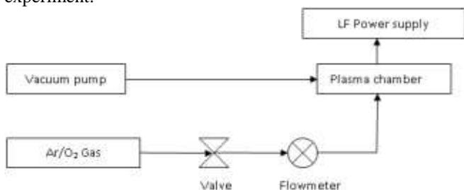
Fig. 2 Flow chart of the plasma treatment set-up
