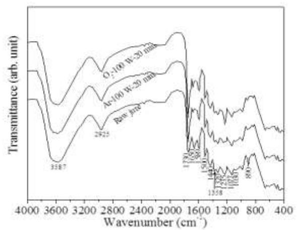
Fig. 9 FTIR spectra of raw, Ar and O<sub>2</sub> LTP treated jute at 100 W, 20 min.
