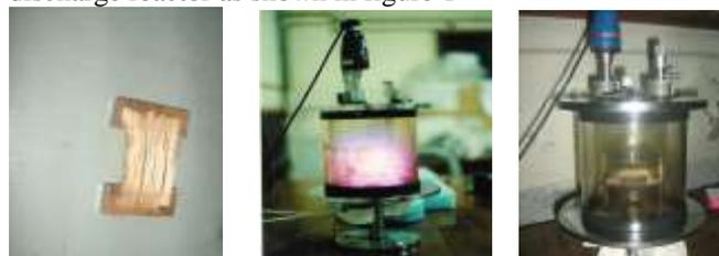
Fig. 1 Schematic diagram of jute fibre and position of it in the glow discharge reactor
