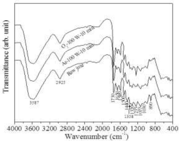
Fig. 7 FTIR spectra of raw, Ar and O<sub>2</sub> LTP treated jute at 100 W, 10 min.
