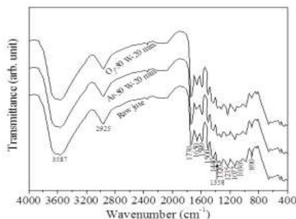
Fig. 4 FTIR spectra of raw, Ar and O<sub>2</sub> LTP treated jute at 50 W, 20 min.
