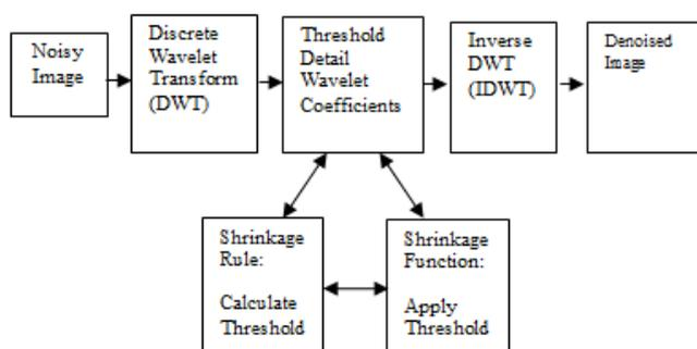
**Fig. 1.** Block diagram of Wavelet-based Image Denoising Method
