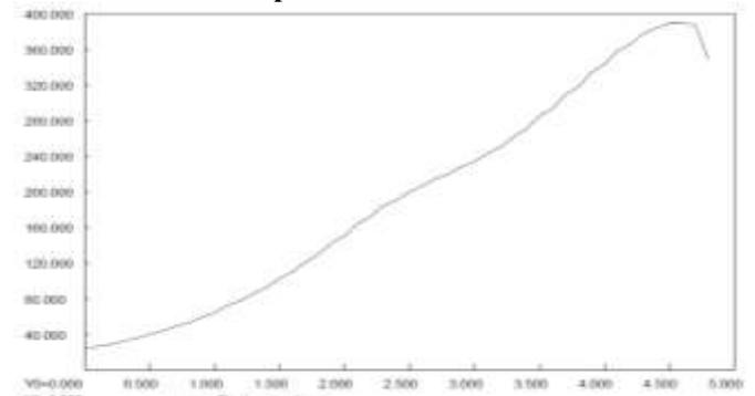
Fig 11: Load Deflection Curve for Steel Reinforced Column
