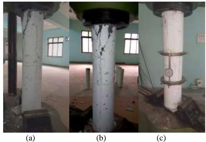
Fig 10: (a) Failure of 100% GFRP Column (b) Failure of Partial GFRP Reinforced Column (c) Failure of Conventional Steel Column
