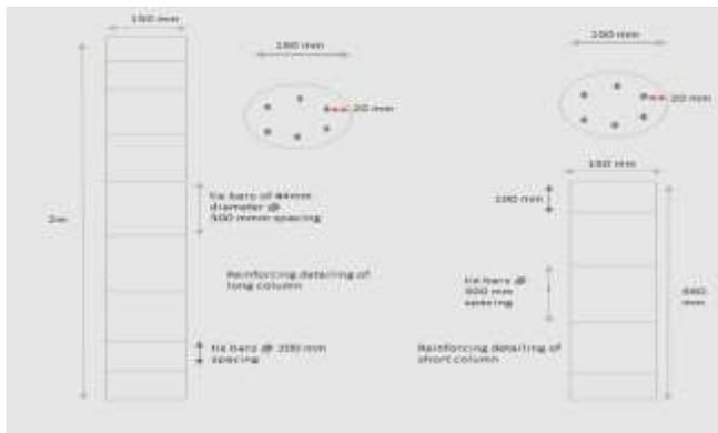
Fig 1: Showing Reinforcing Detailing of Long & Short Columns
