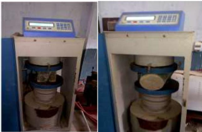
Fig 5: Showing Compression Test of Cubes under & Cylinder
