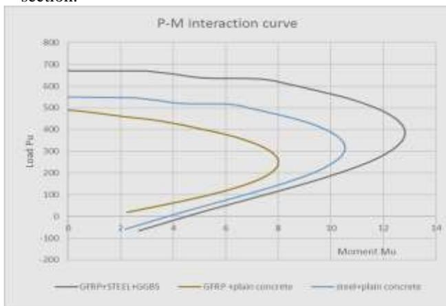
Fig 9: Combined Moment Interaction Diagrams for GFRP Rebar and Steel Rebar of Circular Cross- Section
