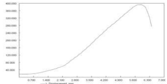
Fig 12: Load Deformation Diagram for GFRP + Steel Reinforced Column
