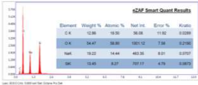
Figure 9. elemental analysis of silica sand waste by EDS spectrometer
