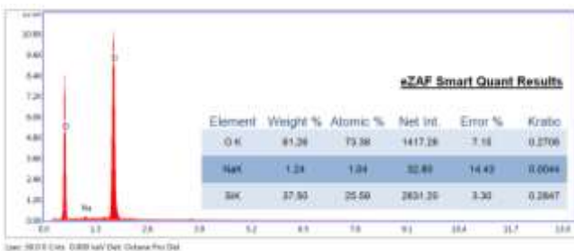
Figure 10. elemental analysis of reclaimed silica sand after third washing by EDS spectrometer
