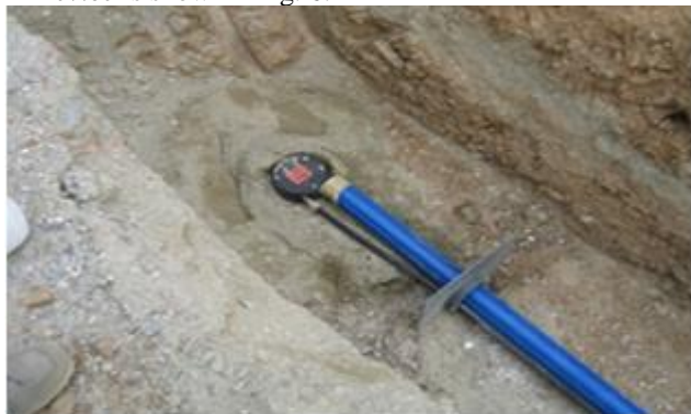
Fig. 6: Horizontal Movement Gauge
