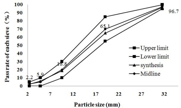
Fig.1. The composite grading curves of recycled aggregate
