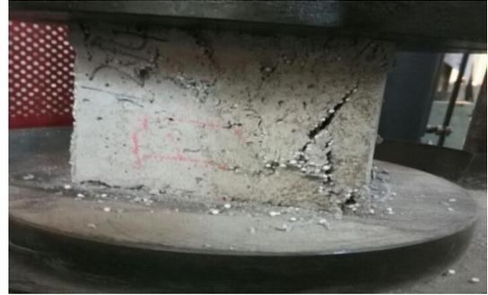
Fig.4.Cube compressive Failure
