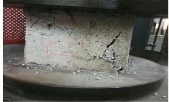
Fig.4.Cube compressive Failure
