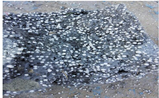
Fig.5.Failure interface of recycled aggregate concrete destruction of the interface between the cement mortar and the EPS particles, and less the interface failure between the aggregate and the fresh cement mortar. The specimen is in a state of unconfined compression so that the edge of the test piece is pulled away to form a penetrating seam, and the interface destruction morphology is as shown in Figure 5.
