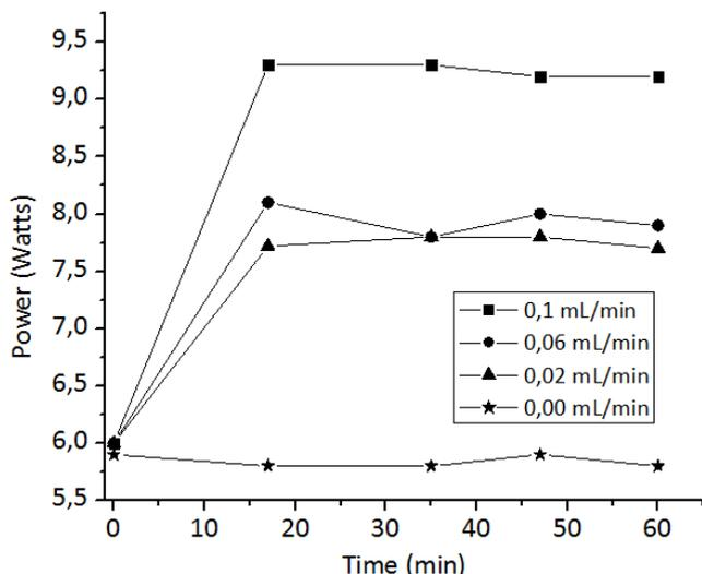
**Figure 6:** Monitoring the discharge power during the reaction time. Experimental conditions: CH<sub>4</sub>/CO<sub>2</sub>=2.3, gas flow: 40mL/min (75% of He), Frequency=5 kHz
