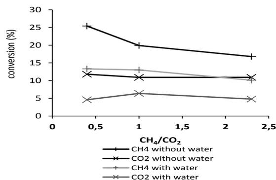
Figure 2: Effect of CH<sub>4</sub>/CO<sub>2</sub> ratio and liquid water (0.06 ml/min) on reactant conversion, gas flow: 40mL/min (75% of He), P=6W
