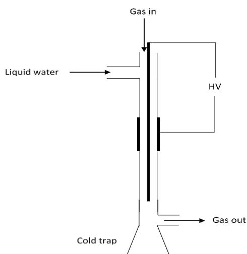
Figure 1: Schematic of the DBD plasma reactor
