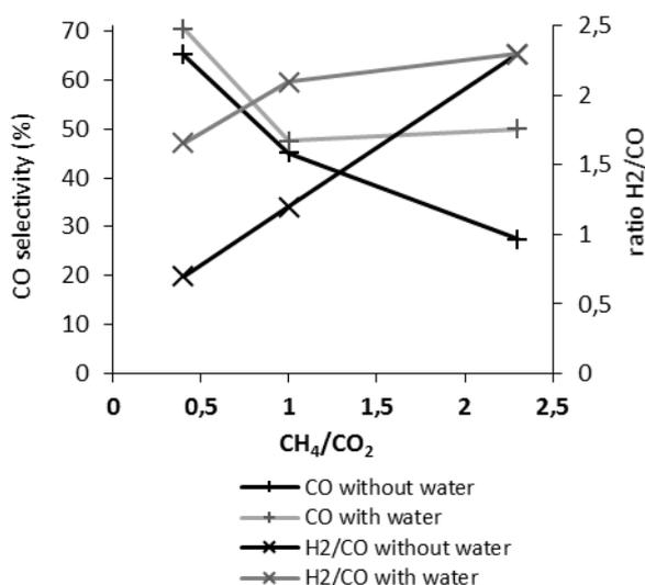
**Figure 3:** Effect of CH<sub>4</sub>/CO<sub>2</sub> ratio and liquid water (0.06 ml/min) on selectivity to CO and H<sub>2</sub>/CO ratio, gas flow: 40mL/min (75% of He), P=6W
