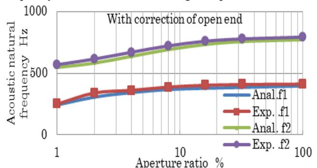
Fig.2 Comparison of Experimental Result with Analytical One
