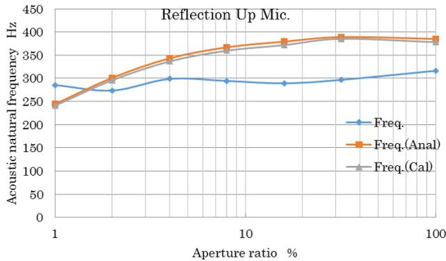
Fig.10 Comparison of Natural Acoustic Frequency Obtained by various Approaches (in the Case of Closed End)
