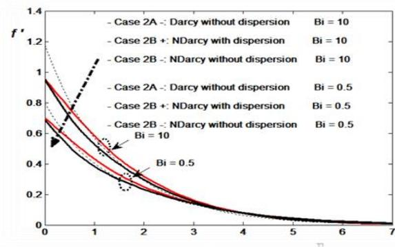
Figure 2: Velocity profile,  $N_b=0.2, N_t=0.1, N_c=0.2, N_r=0.2, L_e=10.0, L_n=10.0$
