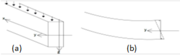
Fig.2 Simply Supported Girder Section and Cross Section Distortion
