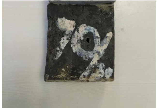
Figure 8. 70% LDPE plastic beads + 30% fly ash bricks
