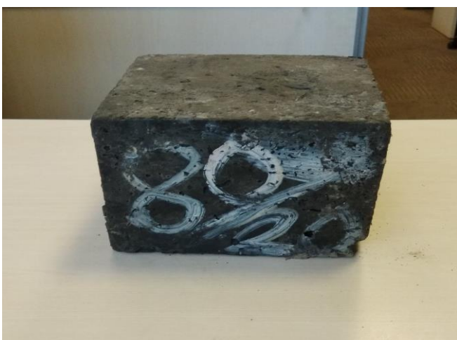
Figure 7. 80% LDPE plastic beads + 20% fly ash bricks
