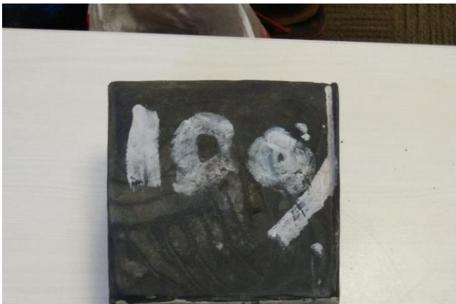
Figure 5. 100% LDPE plastic beads bricks
