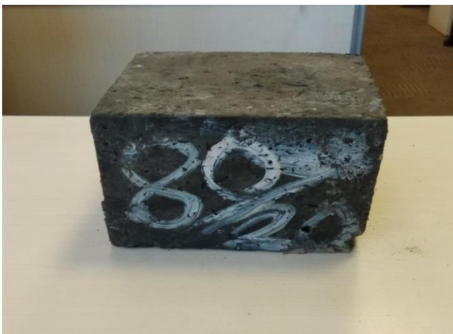
Figure 7. 80% LDPE plastic beads + 20% fly ash bricks
