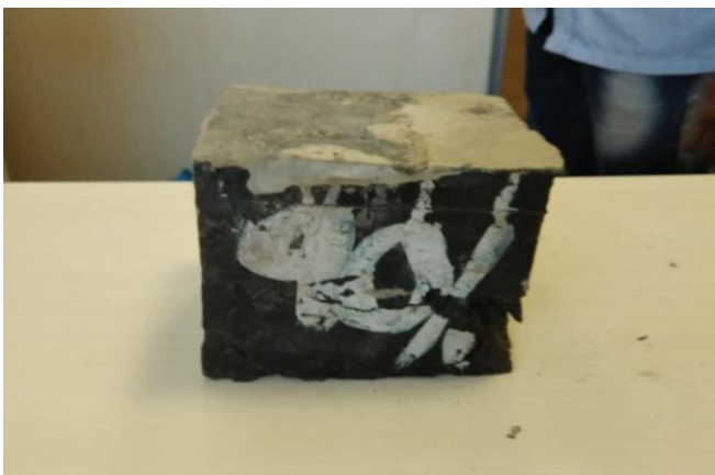
Figure 6. 90% LDPE plastic beads + 10% fly ash bricks
